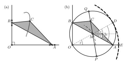
Fig. 3.15. Van Schooten's ellipse-drawing triangle machine
